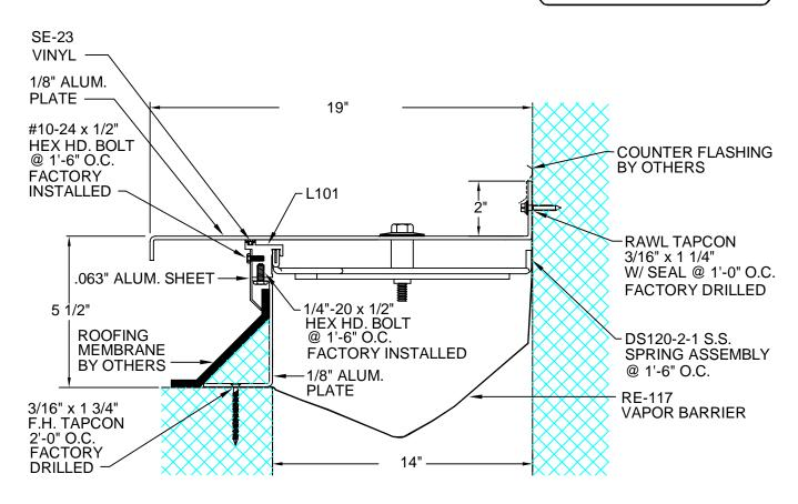
DESCRIPTION: EXTERIOR CORNER ROOF/WALL ALUMINUM: 6063-T5 EXTRUSION, 6061-T6 PLATE
