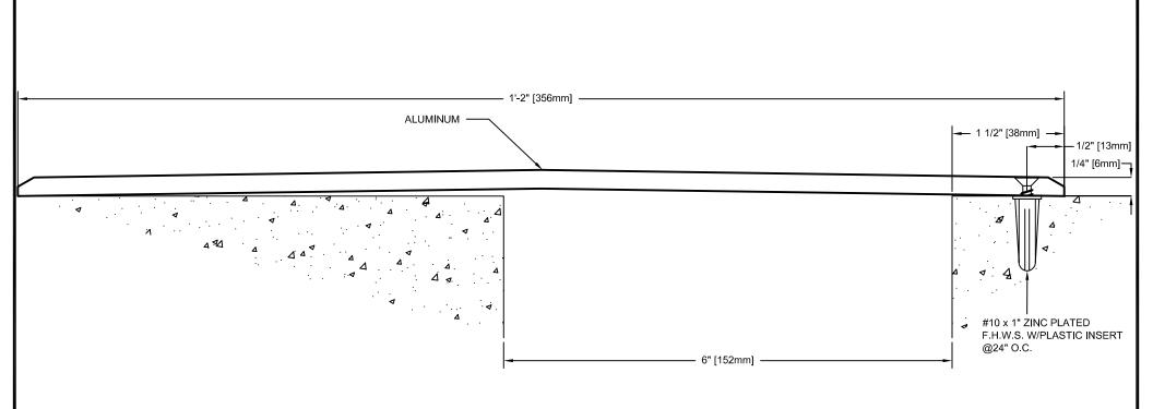
DESCRIPTION: FLOOR-TO-FLOOR ALUMINUM: 6061-T6 EXPOSED FINISH: MILL ALLOWABLE LOAD: CALL FACTORY: 800-835-0028 MOVEMENT: +/- 100 % JOINT WIDTH
