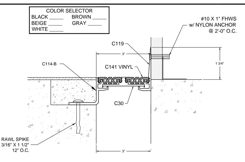
DESCRIPTION: FLOOR-TO-WALL ALUMINUM: 6063-T5 EXTRUSION
