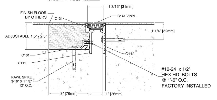
**DESCRIPTION: FLOOR-TO-FLOOR ALUMINUM: 6063-T5 EXTRUSION**
