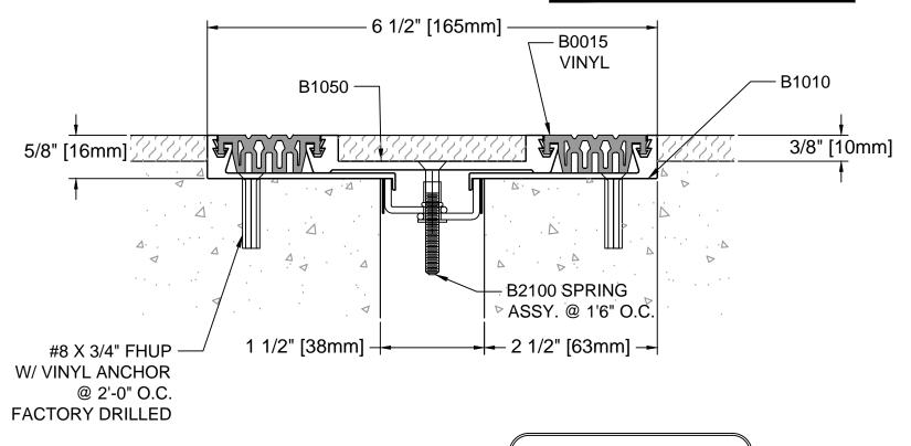
DESCRIPTION: FLOOR-TO-FLOOR ALUMINUM: 6063-T5 EXTRUSION
