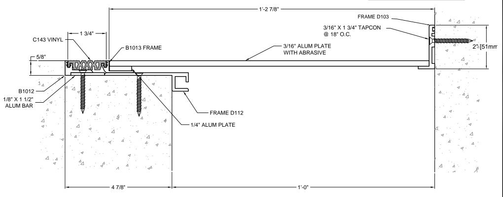
DESCRIPTION: FLOOR-TO-WALL ALUMINUM: 6063-T5 EXTRUSION
